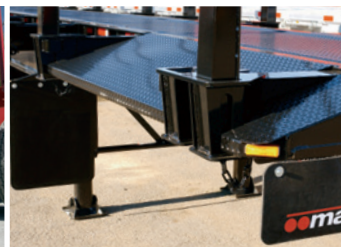
Double pockets for full length wood loads
