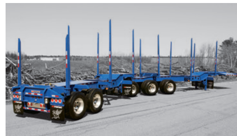
Double pockets for full length wood loads
