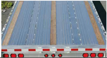
Variety of aluminum structural floor configurations with wood nailers
