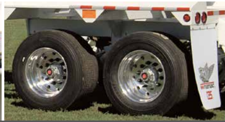
Super single tires with aluminum wheels
