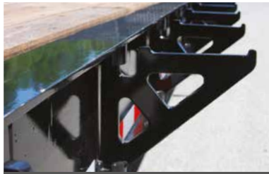
Extensions made of high strenght steel
