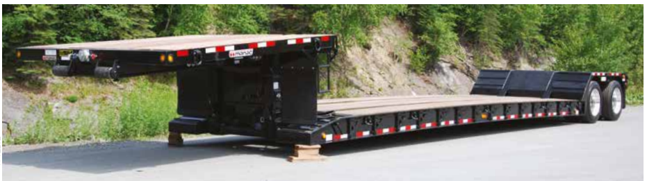
Extensions made of high strenght steel
