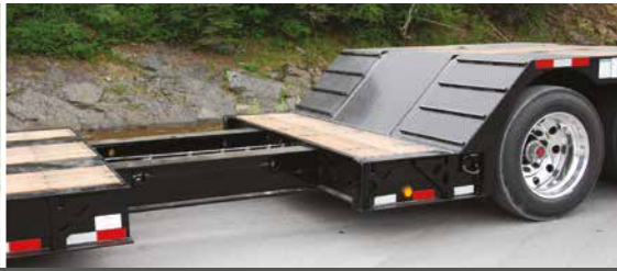
Deck extension with double rollers and air locking pins
