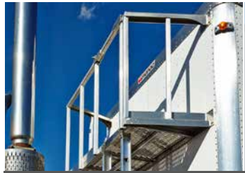
Front catwalk with ladder
