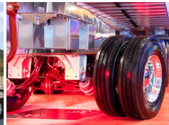
Dual tire on self-steering lift-axle (the only manufacturer offering a real 20° self-steering)
