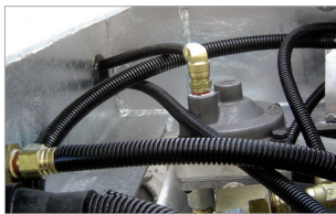
Wire Loom protects air and electrical lines
