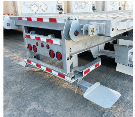
Forklift Package: Offers a removable tire rest and an adjustable wheel stop to accommodate various forklift models.
